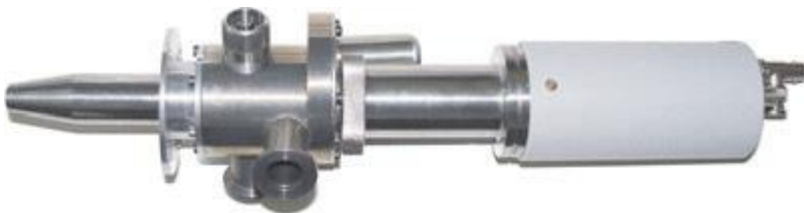
Fig. 4. Scintillation SE detector for VPSEM (total length of detector prototype is 360 mm).
